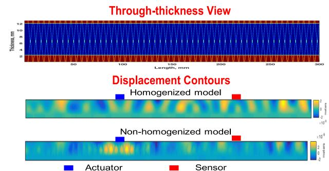
Additional attenuation introduced due to presence of pins **Necessary to consider this effect in SHM for X-COR** sandwich structures
