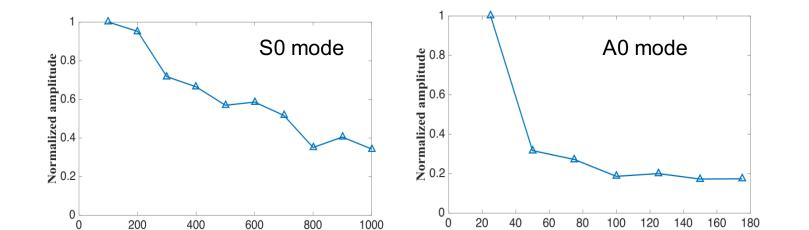
Amplitude decreases with increasing distance away from actuator A0 mode has higher amplitude attenuation than S0 mode
