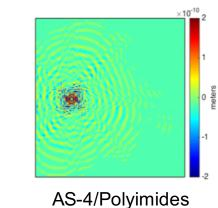
Changing matrix properties do not cause significant change in wave propagation behavior
