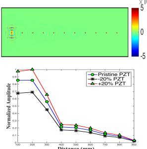
Optimum frequency can be selected based on the functional relation with amplitude Increasing PZT properties leads to higher wave amplitude
