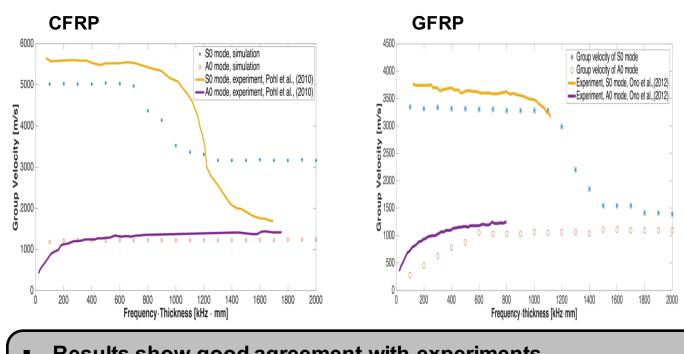
Results show good agreement with experiments The discrepancy of S0 mode in CFRP is due to the different material properties
