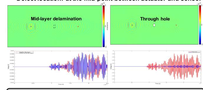
Significant change in wave amplitude due to through hole Wave refection due to damage
