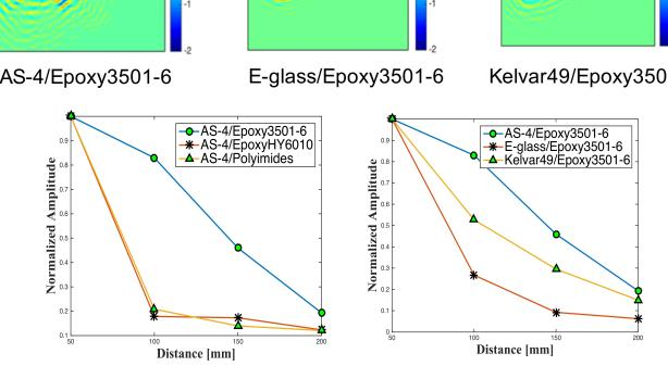
Changes in fiber property lead to significant change in wave propagation
