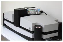
The Micro-CT, an X-Ray 3D imaging machine, was recently added to the AIMS Center Shared Resources. The Micro-CT equipment reconstructs the internal structure and geometry of various material
