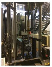
permits a greater variety of loading scenarios such as static and cyclic loading, superimposed tensile and compressive loading, constant and variable amplitude loading, as well as a combination of these options.
