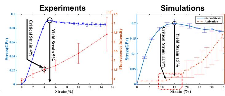
■ Early signal detection of Di-AC was observed in experiments
