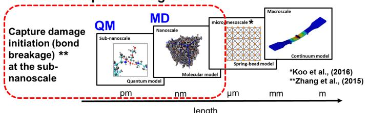
**Quantum Mechanics + Molecular Dynamics** => Hybrid MD Simulation Framework
