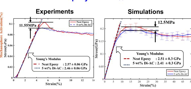
Comparable difference in yield strength between simulations and experiments
