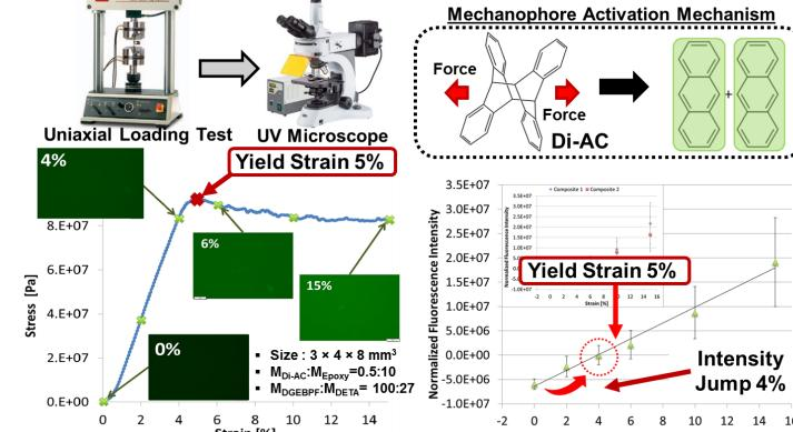
Di-AC nanocomposite successfully shows early signal detection capability
