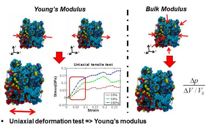
Triaxial deformation test => Bulk modulus
