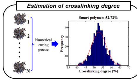
Probability density of crosslinking degree based on a decent number of unit cells with random initial positions of molecules (N=500)
