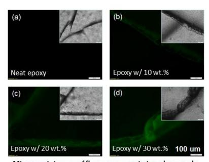
Microscopic images of fluorescence emission along cracks Either TCE polymer coated on polystyrene or blended with epoxy, fluorescence can be observed along crack under UV.
