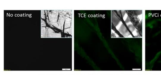
Microscopic images of fluorescence emission along cracks
