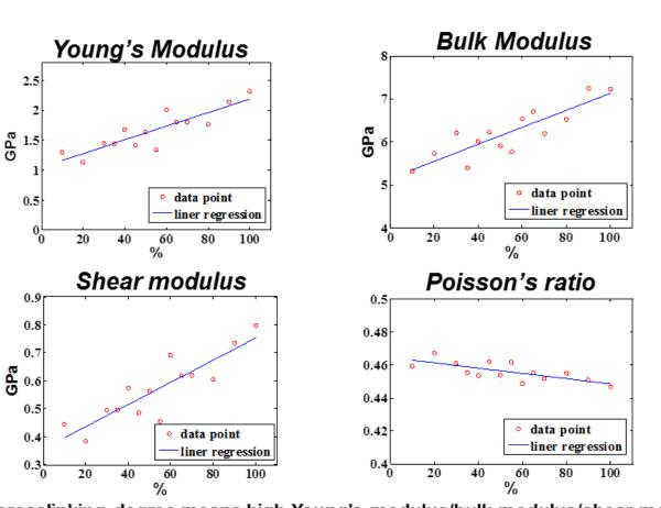
High crosslinking degree means high Young's modulus/bulk modulus/shear modulus. Poisson's ratio are <u>inversely proportional</u> to stiffness of materials
