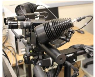
Non-contact full field strain measurement system **Operational through thermal chamber window**
